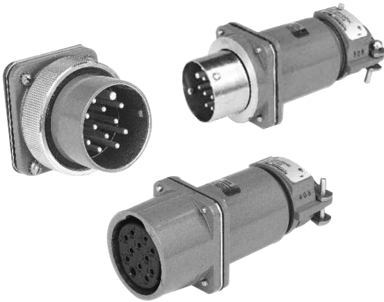
20 A, 250 V AC or DC, 600 V AC maximum rating load-breaking multi-circuit receptacles, plugs, connectors and inlets
