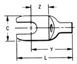
The Type YAV-T-F HYLUG™ is a seamless heavy duty uninsulated compression fork-tongue terminal manufactured from electrolytic copper for use on copper commercial (code) cable, Type AN aircraft cable and extra flexible conductors.
