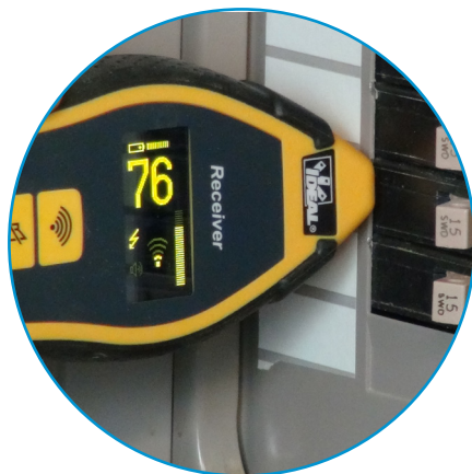
Finding Breakers or Fuses
