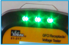
Green Lights Indicate Correct Wiring
