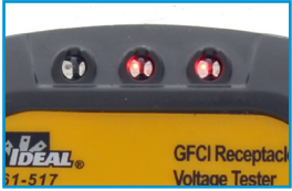
Red Lights Indicate Incorrect Wiring
