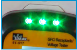
Green Lights Indicate Correct Wiring
