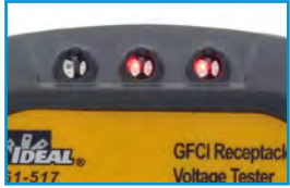
Red Lights Indicate Incorrect Wiring
