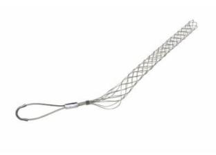
Standard-duty, Closed mesh, Offset eye grips. Cable diameter -1.250-1.490"", Bale length -5"", Mesh length - 15"", Break strength - 1,680lbs.
