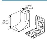
Eliminates need to offset 2400 Series Raceway when connecting with surface panel boxes. Has 3/4" and 1" concentric trade size KOs with 1" trade size KO elongated so adjustment from surface to center of bushing is 1" (25mm) minimum to 1 5/8" (41mm) maximum. Has twistouts for transition to 1500 and 2600 Series Pancake Raceways.
