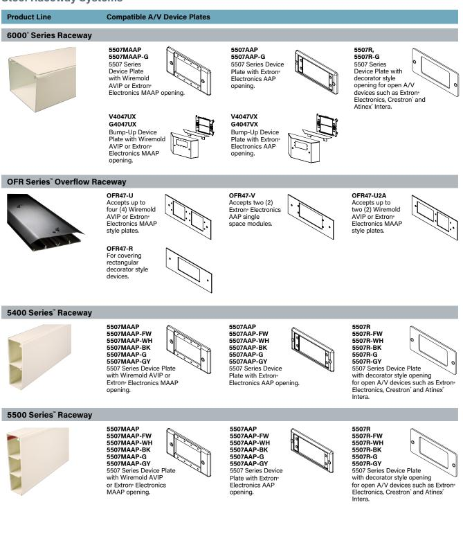
NOTE: Wiremold manufactures many additional pathway solutions. Those represented here have been designed/modified to provide the depth behind the plate required for most A/V devices. For additional design and installation considerations, please contact the factory.
