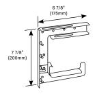
Suspends S4000, 4000 or 6000 Series Raceway from a structural ceiling. Designed for use with 3/8" (9.5mm) rod. Hangers should be installed no more than 5' (1.5m) apart along raceway run. Can be bolted back-to-back for dual runs of 3000, 4000 or 6000 Series Raceway.
