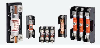
Mersen Class H, K and R fuse blocks accommodate all Class H, K and R 250 and 600V power fuses. A choice of screw, pressure plate, box and special order stud connectors fit a wide range of stranded or solid copper or aluminum wire. Insulators are either molded glass-filled polycarbonate (GFPC) or phenolic with verified dielectric strength in excess of 2500V. 30, 60 and 100A fuse blocks feature a unique adder block which can be snapped onto 1-, 2- or 3-pole blocks to form multi-
