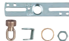
70350 - Brass Finish 70352 - Antique Brass Finish Screw Collar Loop Kit Fits Canopies with a 1 1/8" Center Hole Tapped 1/4"-IP, 35 lb. Load Rating Includes: • 1 Crossbar 4" Long • 1 Screw Collar Loop • 2 Locknuts • 1 Lock Washer • 1 1/4"-IP x 1 1/2" Nipple • 1 3/4"-IP x 1/4"-IP Reducing Hickey • 2 8-32 x 1/2" Mounting Screws
