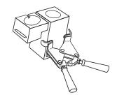
A semi-permanent graphite mold is used for making most Cadweld Connections. The mold controls the direction and speed of the molten Cadweld welding material flow and its final solidified shape. The graphite used in a Cadweld mold is a high temperature type that lasts for an average of 50 or more Cadweld connections under normal usage.
